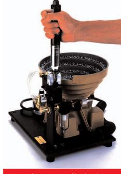
Uniquely engineered bit loader and escapement allow the operator a more ergonomic and natural range of motion.
